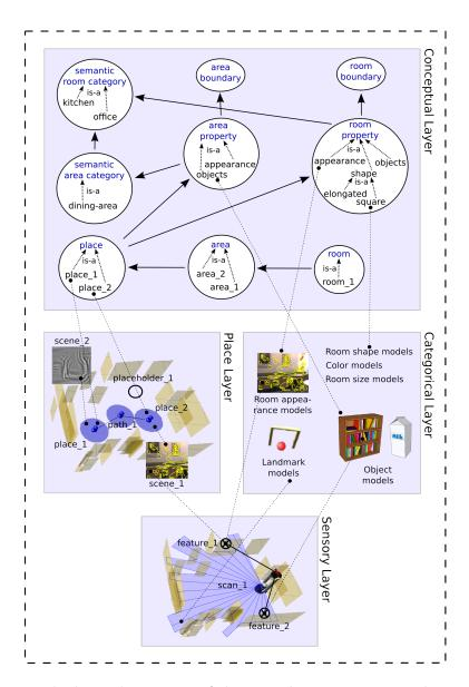
Figure 7: The layered structure of the spatial representation. The position of each layer within the representation corresponds to the level of abstraction of the spatial knowledge.
