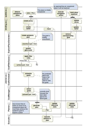
Fig. 13. Activity diagram illustrating the "path" of a knowledge gap from its generation to its filling.
