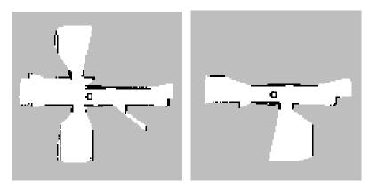
Figure 8: Example of exploration local gridmaps with white: free, black: occupied and grey: unknown space. The position of teh robot is given by the cirtle in the center.
