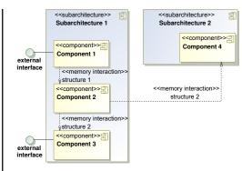
(a) In CAS, there are components, which run in parallel, asynchronously updating shared structures on a common working memory. They can also take input from sensors or give output to actuators. Subarchitectures are coupled to make an overall system.
