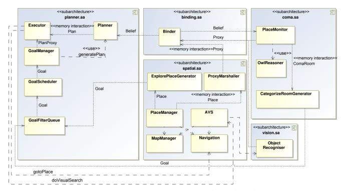
Fig. 10. Dora system architecture. For clarity, all memory interactions are not depicted as information flow mediated through working memories in the subarchitectures but as directed dotted connections of sources and sinks. The dashed lines represent synchronous request-reply calls to components by mutually modifying memory structures.
