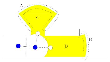
Figure 9: Placeholder creation. Dashed circles are placeholders, each representing one placeholder. A and B are frontier length estimates, C and D are coverage estimates for the respective placeholders.
