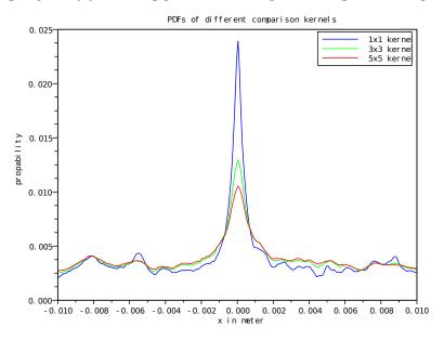
Figure 10: Probability density function of a translational degree of freedom using different levels of observation noise (see text for details)
