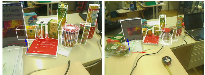
Fig. 9. Good (left) and bad (right) examples of recognition at 0.5 m and 1.0 m respectively, illustrating how recognition performance for some objects degrades with object distance
