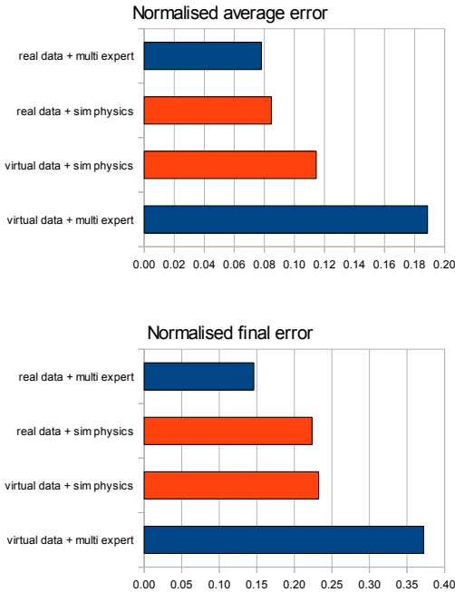
Fig. 9. If only simulation data is available for training of experts, then incorporating a simple physics predictor improves performance, approaching that of the ideal situation in which experts are trained on real observations of real objects. These charts compare the performance of a combination of learned experts which have been trained only on erroneous synthetic data, with and without the incorporation of an additional expert based on simple physics. In each case, performance has been assessed by then attempting to make predictions about motions of real objects which were not seen during training. For comparison, we also show data for the ideal situation in which experts have been exposed to examples of the real object during training.
