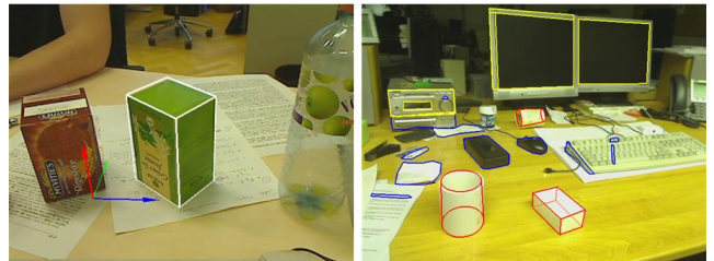
Figure 7: The left image shows a detected textured tea box on cluttered background. The right one illustrates detected object shapes from cubes and cylinders (red) as well as rectangles (yellow) and closures (blue) from lower-level Gestalts in an office scene.
