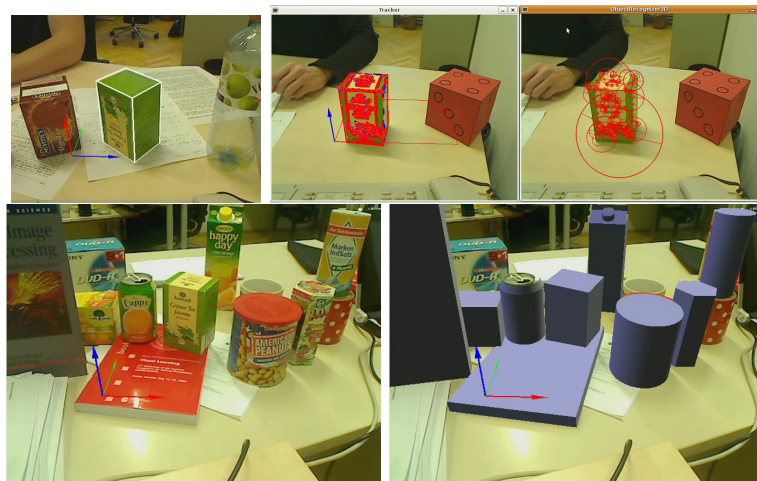
Figure 1: Edge based detection and tracking (top left and center) and SIFT feature on the object (top right). Recognition results for 10 objects (bottom)
