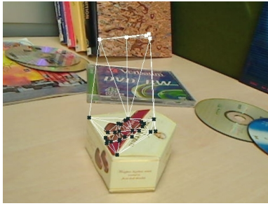
Figure 1: A plane (top surface of packaging) accidentally picks up interest points in the background. Therefore we split the interest point clusters (coloured dots) using the mean and standard deviation of edges of a Delaunay graph (white edges).
