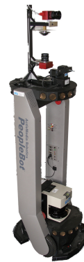
(d) The mobile robot used for acquiring the data. The cameras and the laser scanner can be seen on the top and bottom platforms, respectively.
