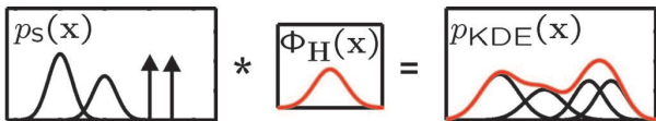
Fig. 2. Calculation of the KDE p_{KDE}(\mathbf{x}) through a convolution of the sample distribution p_s(\mathbf{x}) with a kernel (Dirac-deltas are depicted by upward arrows).
