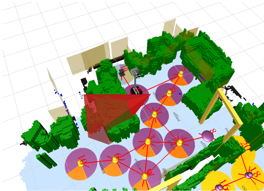
Figure 3: Peekabot visualisation for the Dora system. Obstacles are shown as green blocks. The Places used for planning are shown as pins on the ground, together with the paths connecting them. The “pie charts” around each Place represents the confidence in various classifications of the room in question. Blue dots and beige rectangles show laser scans and SLAM line features, respectively, while a red pyramid shape represents a view cone used to search for an object. Each component in the system can contribute its own visualisation independently.
