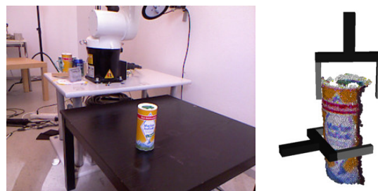
Fig. 10: Grasping a novel object using a dictionary of parts. The rightmost image shows the grasps suggested by the first and last prototypes of Fig. 9, respectively approaching the object from the side and from the top.
