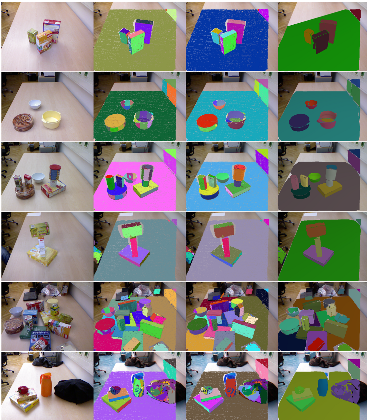
Figure 4. Selected examples of the proposed approach. The first column shows the color image, the second one the estimated planes, the third the plane patches and NURBS after model selection, still as point cloud. The last column shows the segmented object models.
